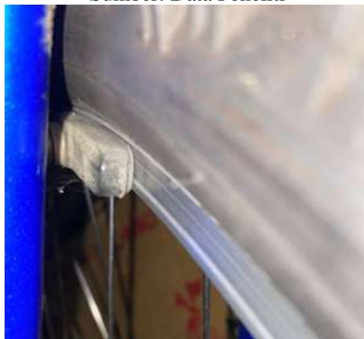
Gambar 2. Bantalan Rem Sepeda Yang Menjepit Pelek Roda Sepeda Saat Direm
